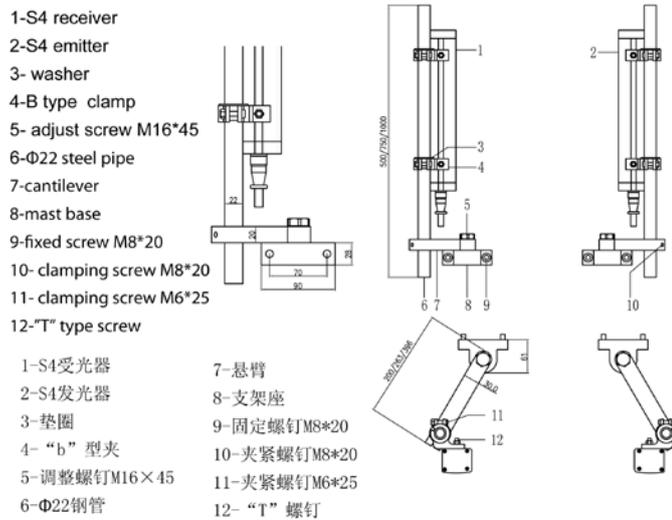
Figure 4-5 Installation of split steel pipe brackets
