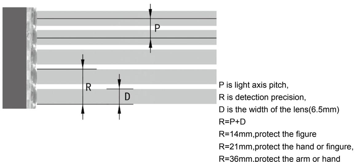
Figure 2-1 Relations between light axis pitch and protection object
