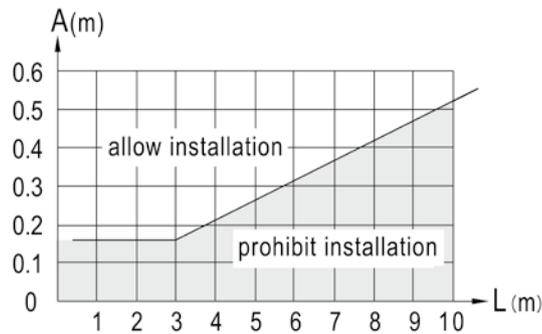
Figure 4-4 The placement position schematic drawing of prevented the influence from the reflecting surface around the light curtain
