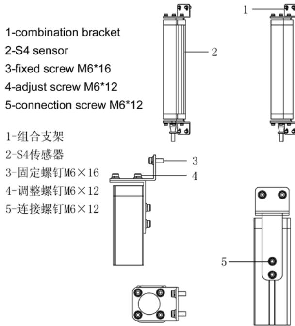
Figure 4-7 Installation of combined brackets
