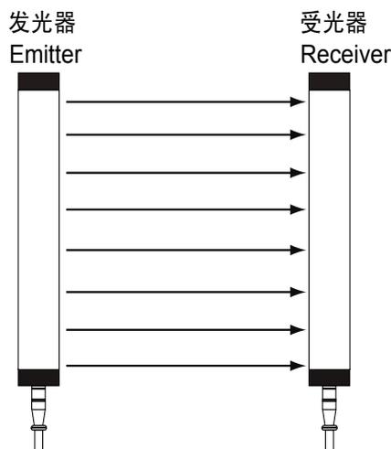
Figure 2-2 Working schematic drawing of S4 series
