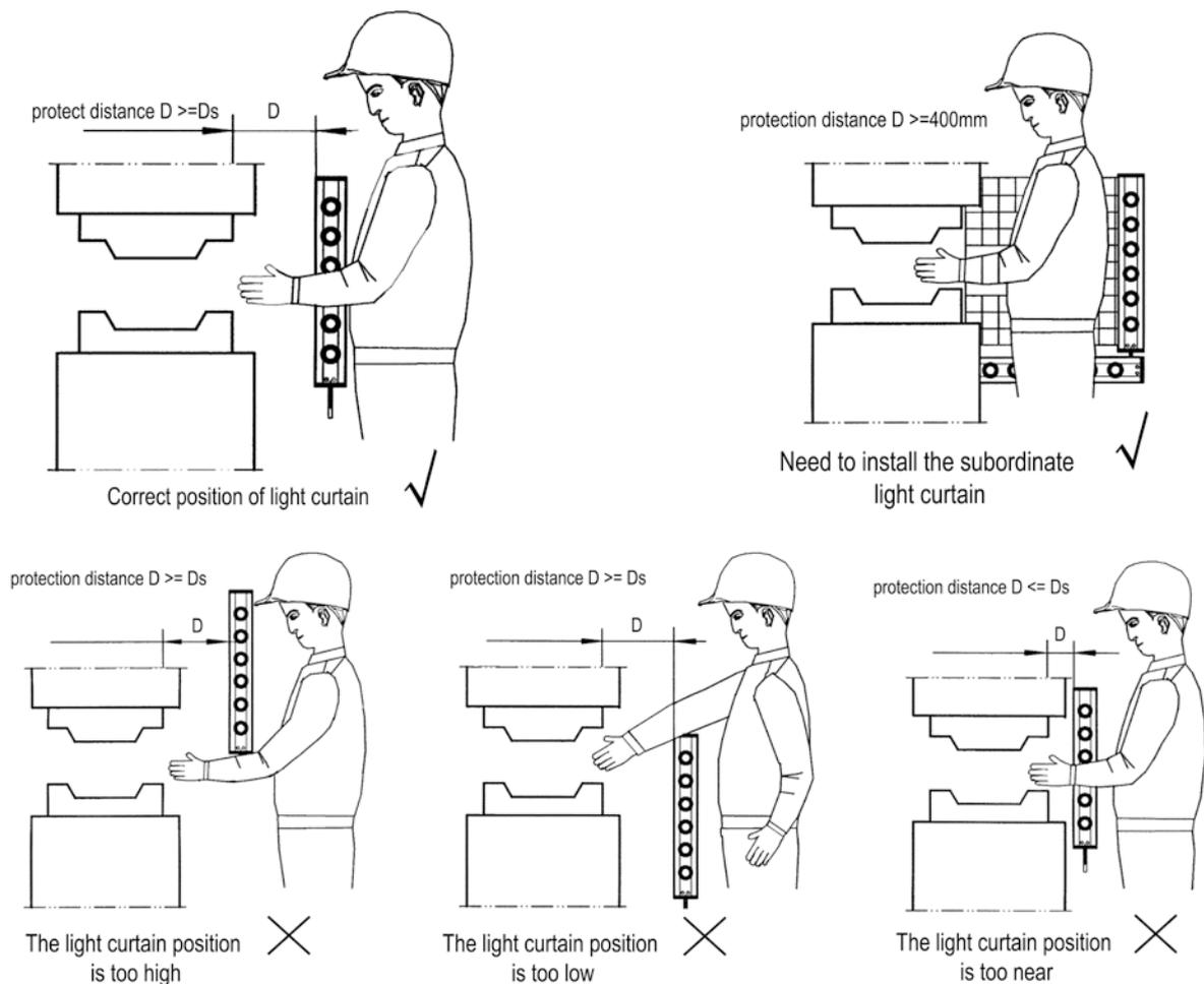
Figure 4-2 Placement position schematic drawing for light curtain
