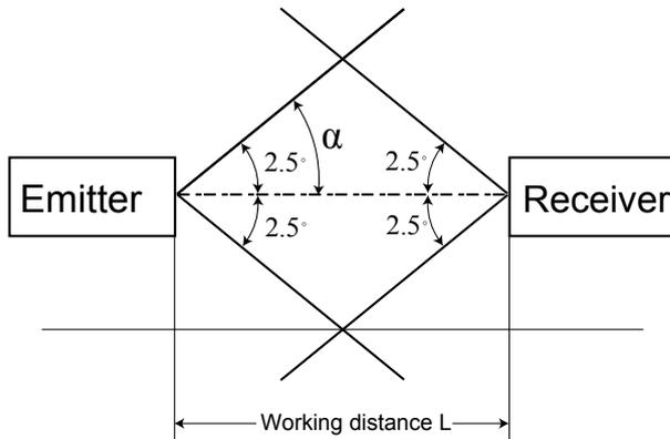
The cone has a aperture Angle alpha, it formed between the optical axis and a light beam on the edge of the cone.
