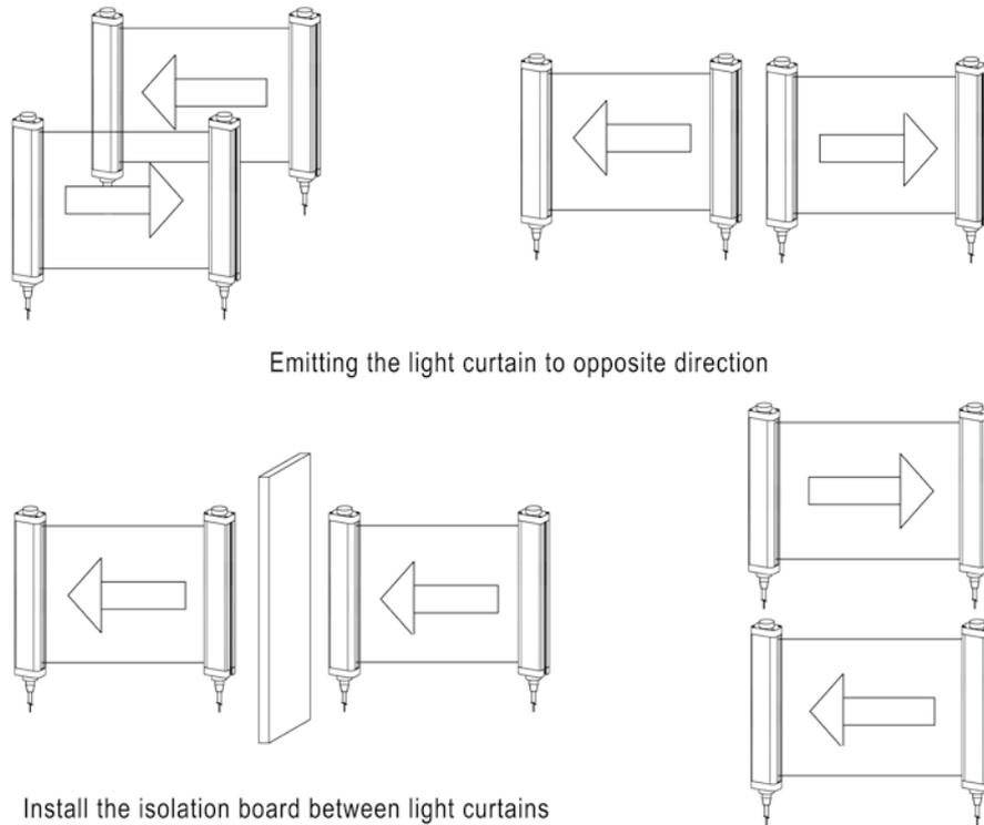
Figure 4-3 Placement schematic drawing for prevented the neighboring light curtain disturbs mutually
