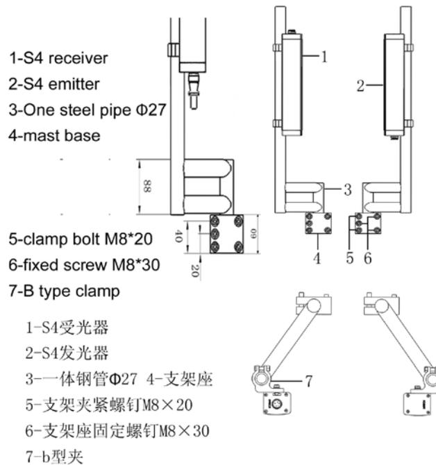
Figure 4-6 Installation of integrated steel pipe brackets
